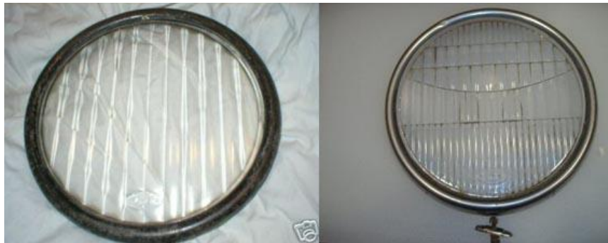
Comparison of Model A Headlight Lenses 1928 Lens (left) has vertical "flutes" - 1929-1931 Lens has different design Both have the Ford Script in an oval at the bottom of the lens
